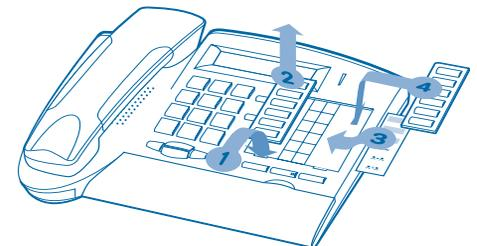
1. Insert a flat “blade” into the slot (1 slot per key block).
